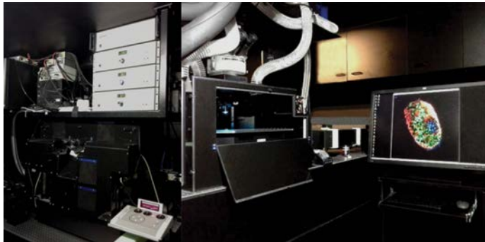
Figure 2 Two-photon excitation microscopy system: view of inverted and upright microscopes.
